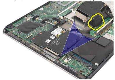
CAUTION: Incorrect installation of the rubber bumper may damage the hard-drive flex cable.
