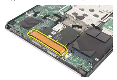
4 If installed, remove the cloth tape on the edge of the card-reader board.
