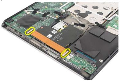
**3** Gently peel the hard-drive flex cable away from the system board.
