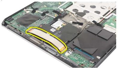
**9** Press the hard-drive flex cable to ensure that the double-sided tape sticks to the edge of the card-reader board.
