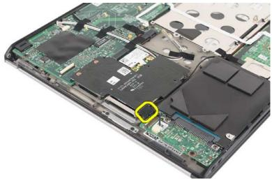
**5** Peel the double sided tape on the rubber bumper (shipped with the hard-drive cable kit) and install the rubber bumper as shown in the figure below.
